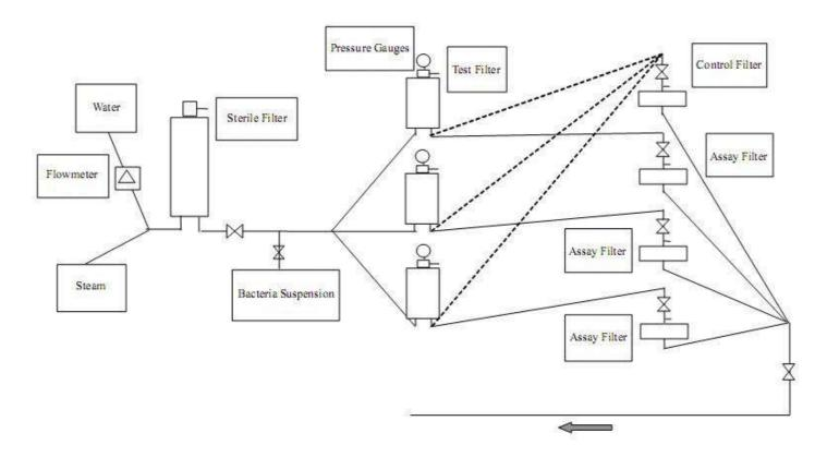
PES 0.45µm filter with different batch lots were subjected to microbial challenge tests using an aqueous suspension of *Serratia marcescens* (ATCC 14756).
