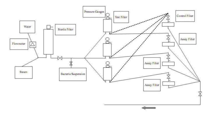
Double Layer Hydrophobic PTFE 0.2+0.2µm filter cartridges with different batch lots were subjected to microbial challenge tests using an aqueous suspension of *Brevundimonas diminuta* (ATCC 19146).
