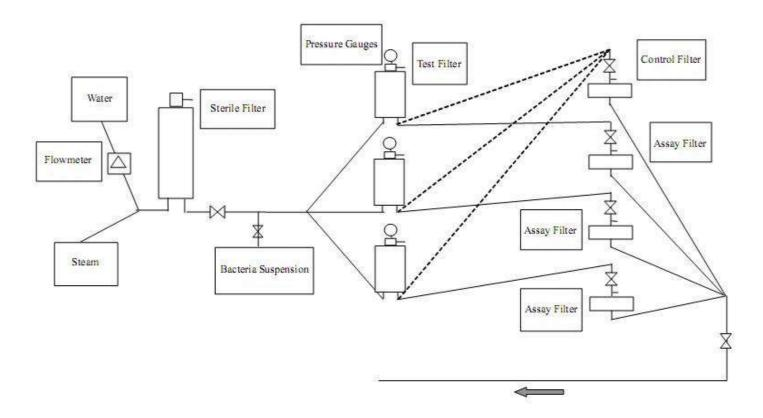
Double layer PES 0.45+0.2µm filter cartridges were subjected to microbial challenge with different batch lots tests using an aqueous suspension of *Brevundimonas diminuta* (ATCC 19146). Prior to the challenge tests the filters were installed in an appropriate housing, flushed with DI water at a flow rate of 4 L/min for 15~20 minutes, and then autoclaved at 121 °C for 30 minutes. The filter assembly was then aseptically connected to a pre-sterilized challenge apparatus.
